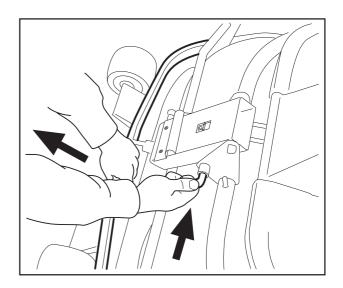
9. Grasp the front edge of the cutting unit, pull out and raise into the service position.
